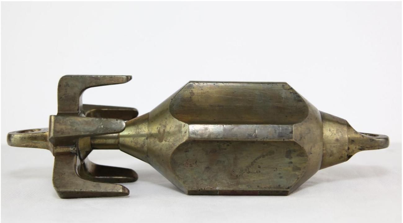
**Our object of the week is a small solid brass model of a Murphy grapnel. The Murphy grapnel was used for locating and picking up cable from the seafloor. The grapnel was an indispensable part of cable repair ship equipment and there were dozens of different types. There were grapnels for rocky bottoms, others for sandy (much like our Porthcurno coastline), and chain grapnels which were similar to a length of hefty chain with hooks along its length.**
